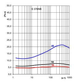
Paste preparations with 40, 50 and 55 phr DINP. Readings were made 1 h after preparation at 23 °C with rotating and capillary viscosimeters.
