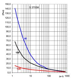
Paste preparations with 85, 100 and 120 phr DINP. Readings were made 1 h after preparation at 23 °C with rotating and capillary viscosimeters.
