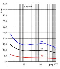
Paste preparations with 50, 55 and 70 phr DINP. Readings were made 1 h after preparation at 23 °C with rotating and capillary viscosimeters.
